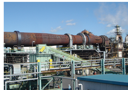
JX Nippon Tomakomai Chemical rotary kiln furnace
