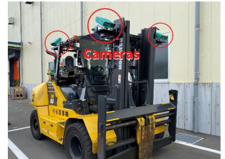
Intelligent cameras installed on forklifts
